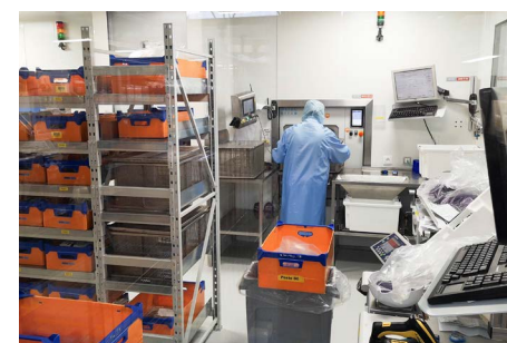
ISO 7 cleanroom packaging Château-Gontier-sur-Mayenne, France
